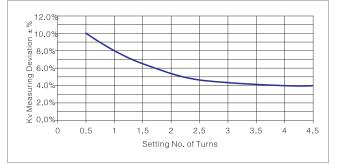
Accrding to the standard, When the valve's opening rate is greater than 50%, the deviation is lower than  $\pm 5\%$ . Based on this, it is suggested to choose a valve with at least 50% opening rate when working under the design flow. Additionally, in order to ensure adequate on-site commissioning allowance. It is recommended to set the valve at around 75% opening rate.
